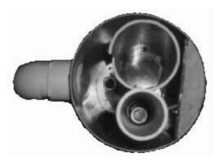
Figure 16. Top view of side stream sampling device. Note the location of the baffle and bottom drain in relation to the debubbler and instrument deployment tube.
