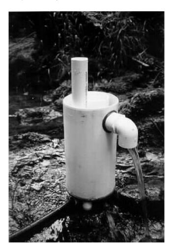
Figure 15. Side stream sampling device being tested.
