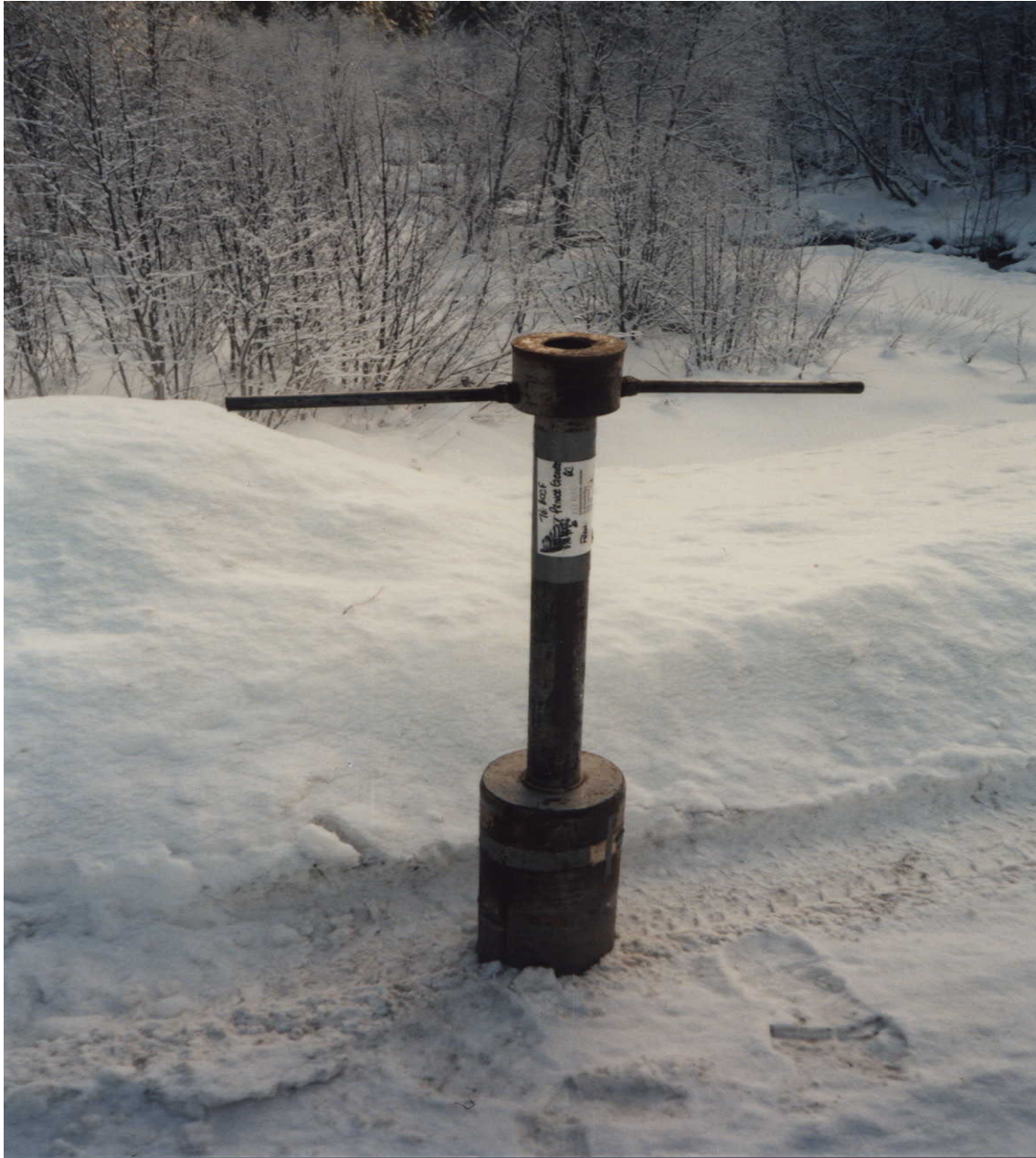
Figure 4 – Roadside photo of the modified freeze corer outer tube, which standardizes the volume of sediment that can be sampled (Rood and Church, 1994).
