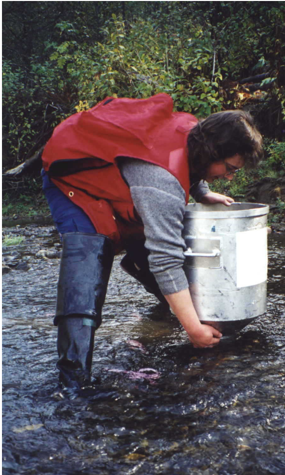
Figure 10 - To ensure that the core is fully inserted, the sample basin should be flush with the streambed.
