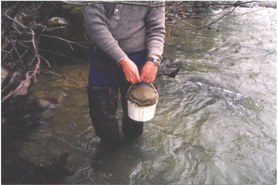
Figure 17 - Overfilled gravel bucket. This sample can only be used qualitatively because the effective sample period is not known.
