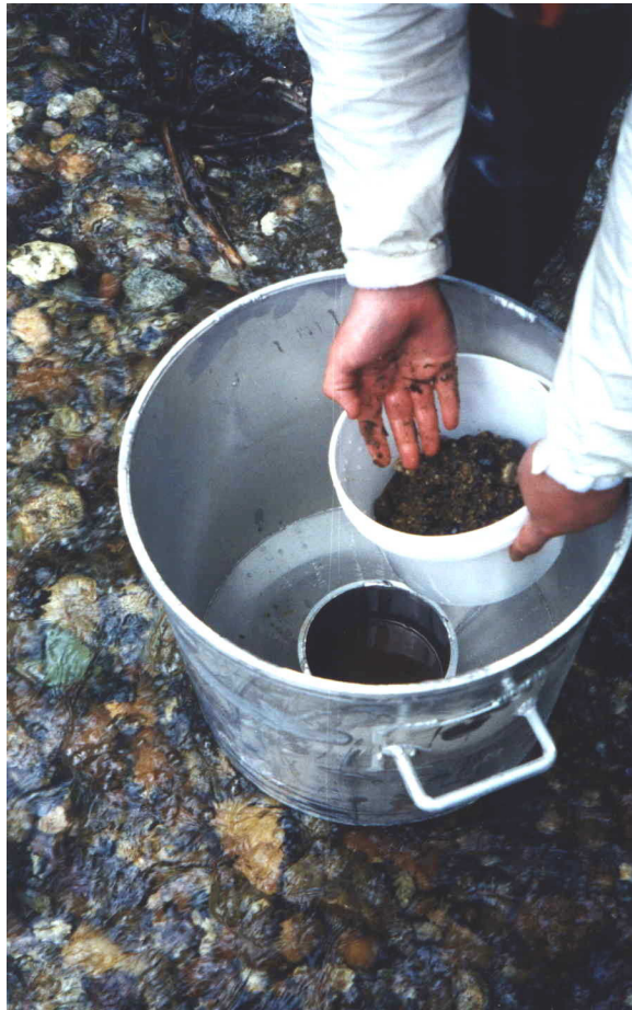
Figure 11 - Sediment removal from core tube directly into 4 -litre bucket. Note: water has not entered the sample basin and grit on the sampler's hand was washed off into the sample bucket.
