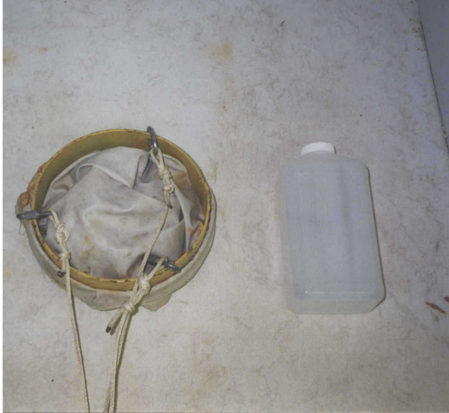
Figure 18 - Infiltration bag, top view into ring with collapsed bag. (1 liter sample bottle for scale)
