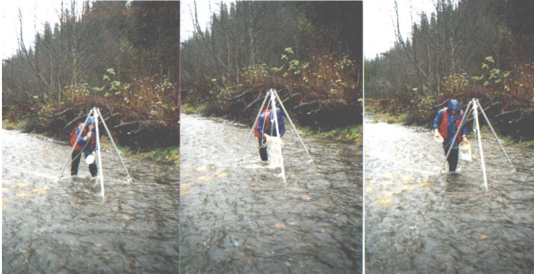
Figure 20 - Infiltration bag removal by a sole staff member. Photos left to right: tripod's pulley system is used to bring bag up through reference gravel to streambed surface, the bag is capped and removed from the streambed, and brought to processing area.
