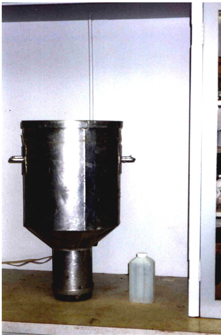
Figure 6 - Modified McNeil core design. (1 liter bottle for scale)
