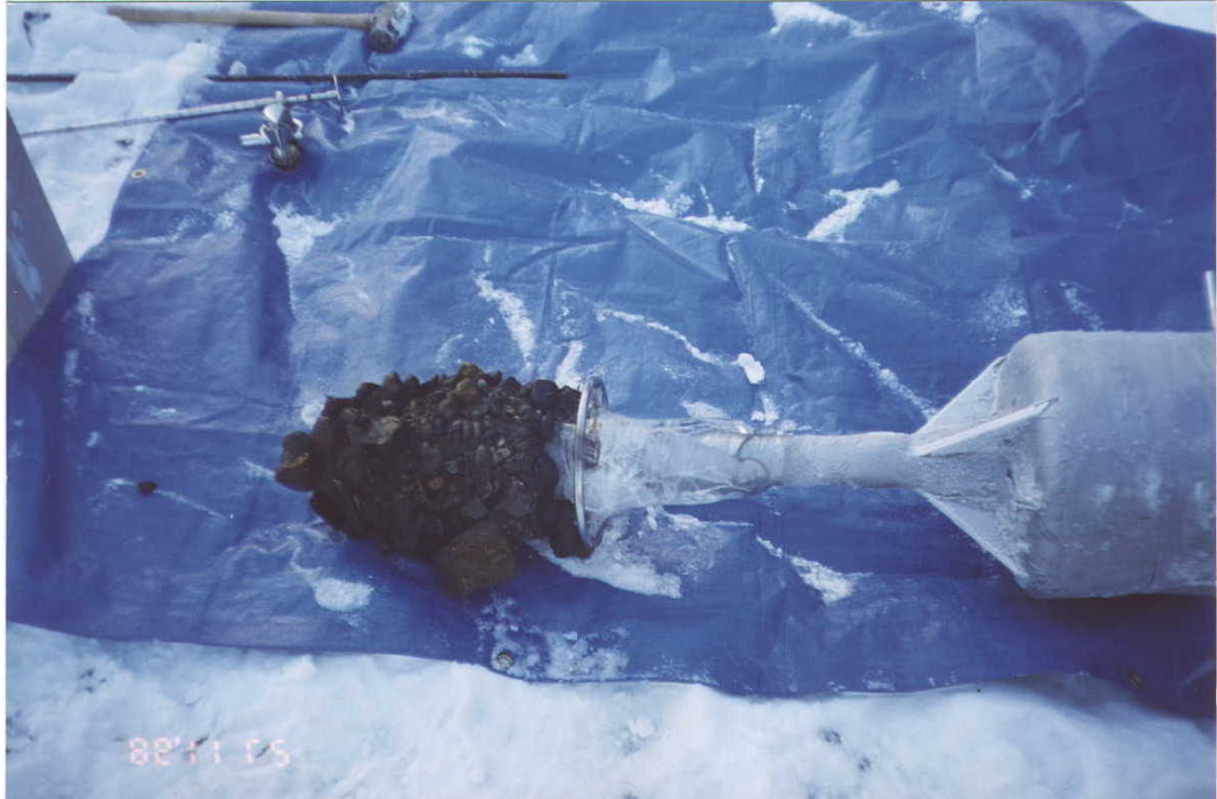
Figure 2 - Single probe freeze corer. (Photo courtesy of Jessy Harper, Agra Earth & Environmental).
