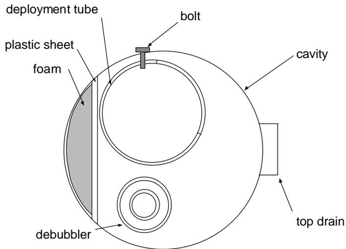
Figure 14. Plan view of side stream sampling device.
