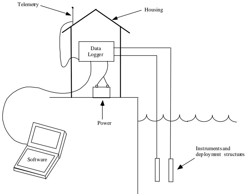
**Figure 3. Components of an automated monitoring system.**
