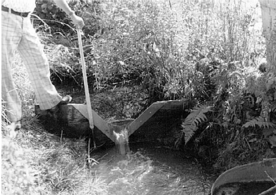
**Figure B-6. V-notch weir, portable installation.**
