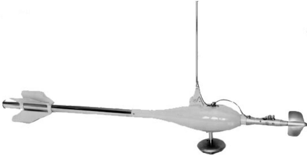
Figure C-25. OSS B1 current meter mounted on a 30-kg sounding weight (middle), with a bottom feeler.
