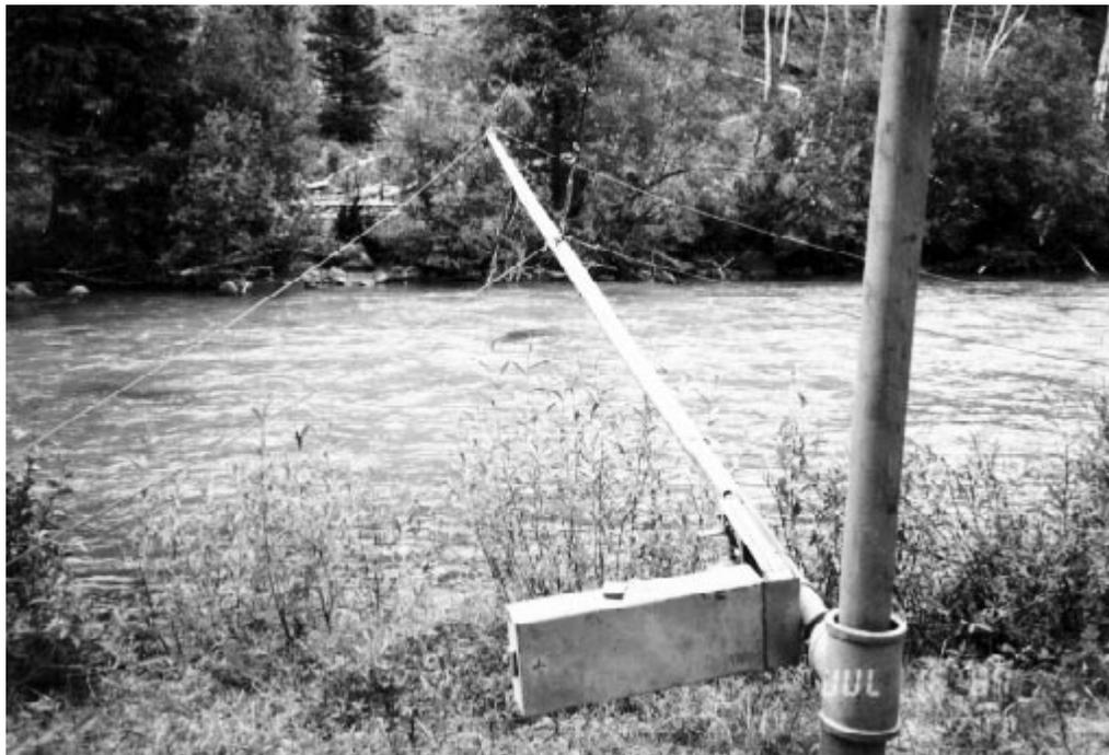
**Figure B-13.** Boom wire weight gauge.
