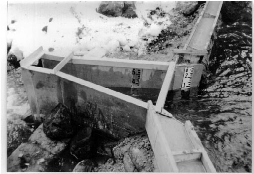
**Figure C-33. Six-inch Montana flume set in permanent concrete sack structure.**
