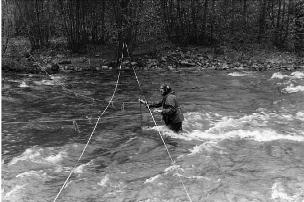
**Figure D-3. Measuring by wading, with safety line angled upstream, Granite Creek near Tulameen.**
