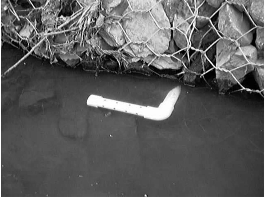
**Figure C-7. Static tube for intakes.**
