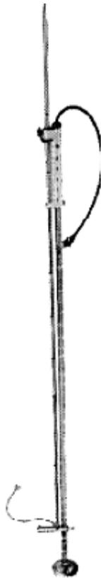
**Figure C-27. Top setting wading rod.**
