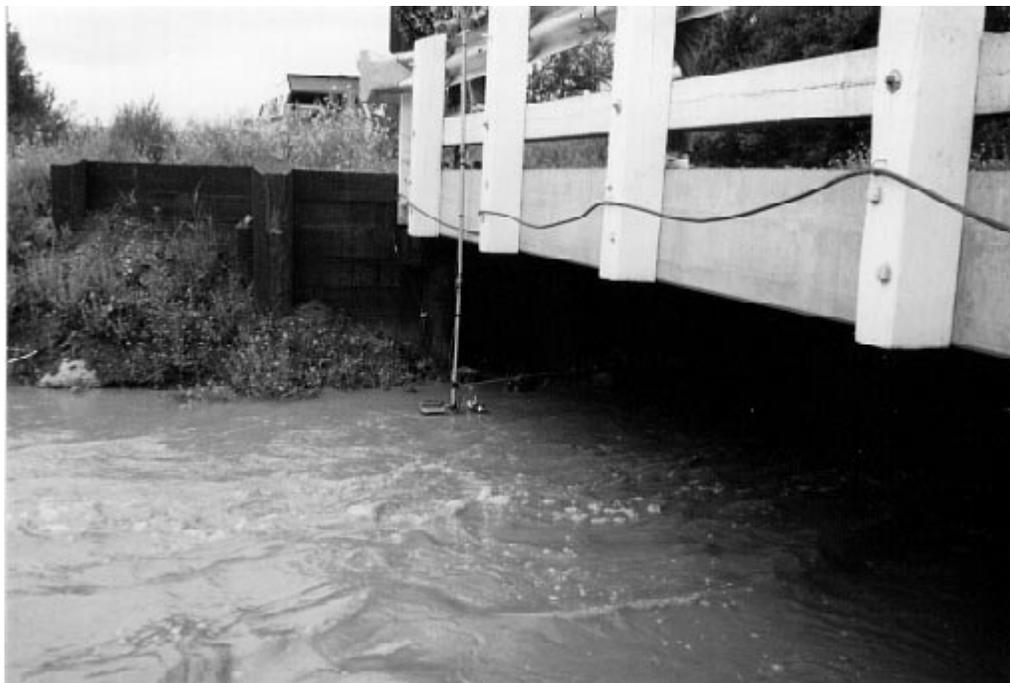
Figure D-8. Bridge rod in use on downstream side of bridge.
