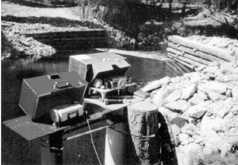
**Figure B-1. Two water level recorders: a data logger and an analogue recorder.**
