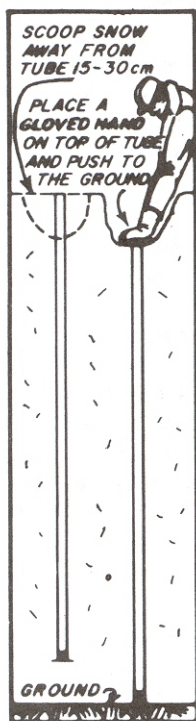
FIG.14a WHEN SNOW DEPTH IS SLIGHTLY MORE THAN LENGTH OF SAMPLING TUBE
